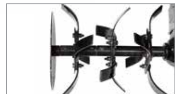
85 cm rotor with lateral protection discs.
