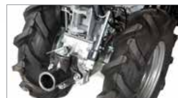
QuickFit coupling that allows the operator to change the tools without using tools.
