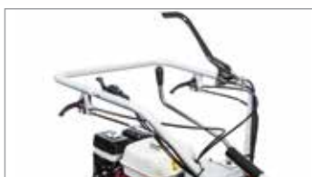
Steering with independently controlled releases and brakes.
