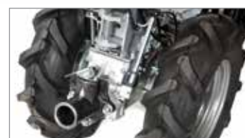
QuickFit coupling that allows the operator to change the tools without using tools.
