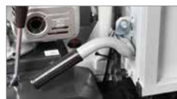
Manual dump with automatic locking system.
