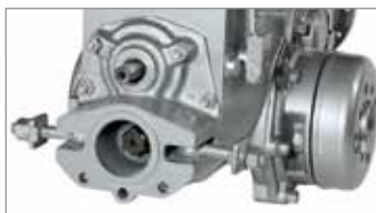
Two power take-offs, one independent two-speed PTO and one synchronised PTO.
