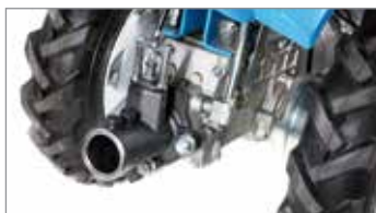
Integral QuickFit coupling that allows the operator to change the tools without using tools.
