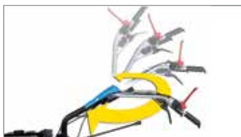
Handlebars with vertical and horizontal adjustment by means of an easily accessible lever, allowing the operator to assume the correct posture for the maximum working comfort.
