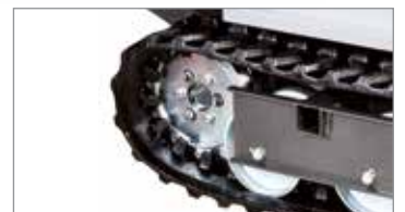
Protected, expandable brakes for working in extreme conditions.
