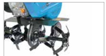
46 cm rotor with three elements per side, can be reduced to 32-22 cm.
