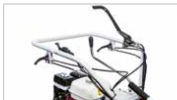
Steering with independently controlled releases and brakes.
