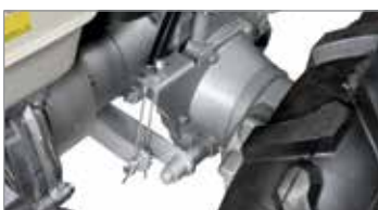
Steering clutches with control in combination with the brakes allow the machine to turn 360° with a minimum turning radius.
