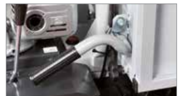
Manual dump with automatic locking system.
