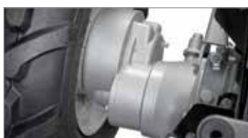
Half-shafts with final reduction gears to improve grip on steep inclines.
