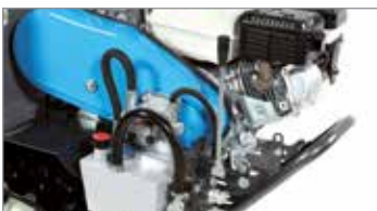
Lever-operated hydraulic tipping control valve.
