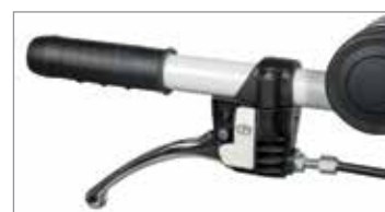
Independently controlled brakes and parking brake.
