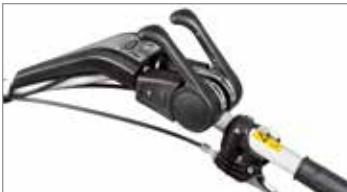
Ergonomically positioned easy action levers for differential locking and reverse shuttle.
