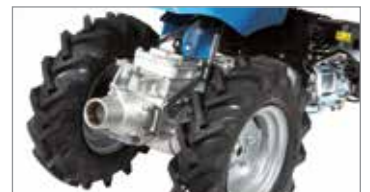
Integral QuickFit coupling that allows the operator to change the equipment without using tools.
