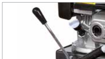
Speed selection control lever.
