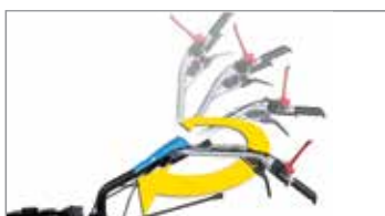
Handlebars with vertical and horizontal adjustment by means of an easily accessible lever, allowing the operator to assume the correct posture for the maximum working comfort.
