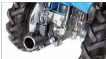
Integral QuickFit coupling that allows the operator to change the equipment without using tools.
