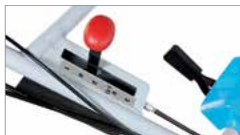
Extreme versatility thanks to the 4-speed gearbox (3 forward + 1 reverse) that makes it possible to achieve the same tillage results irrespective of the hardness and consistency of the soil.
