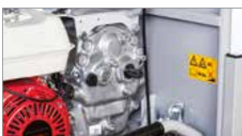
Independent PTO at 2100 rpm.
