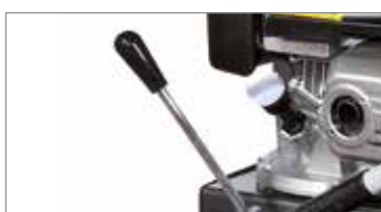
Speed selection control lever.
