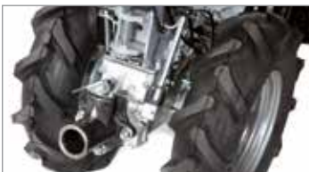
QuickFit coupling that allows the operator to change the equipment without using tools.
