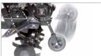
Front wheel for easy transportation of the machine. The wheel can be easily folded upward without tools to facilitate operations on the ground.
