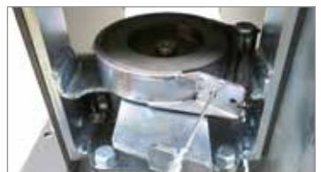
The service and parking brake engages automatically when the clutch is released, to prevent accidental hazardous movements.
