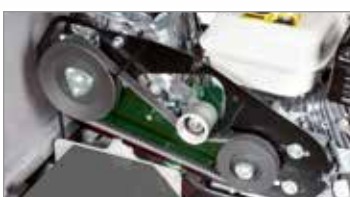
Belt clutch with automatic disengagement when the control lever is released.
